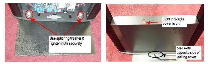
5. Now you are ready to plug in your towers. The Ebony I series has a light at the top of the base (on the Euro model it is on the front cover) to let you know that power is "on". This is so you do not have to take the side cover off to determine if the board is getting power.
